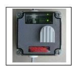
DG-nn.EN/M has an exchangeable module with carbon monoxide, methane, propanebutane or HFC sensor. Interchangeable sensor module streamlines maintenance, simplifies calibration and reduces operating costs.
