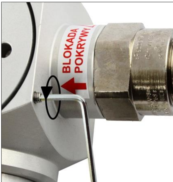
Fig. 3.3. BEFORE unscrewing the cover ==> unscrew the COVER LOCKING screw:
